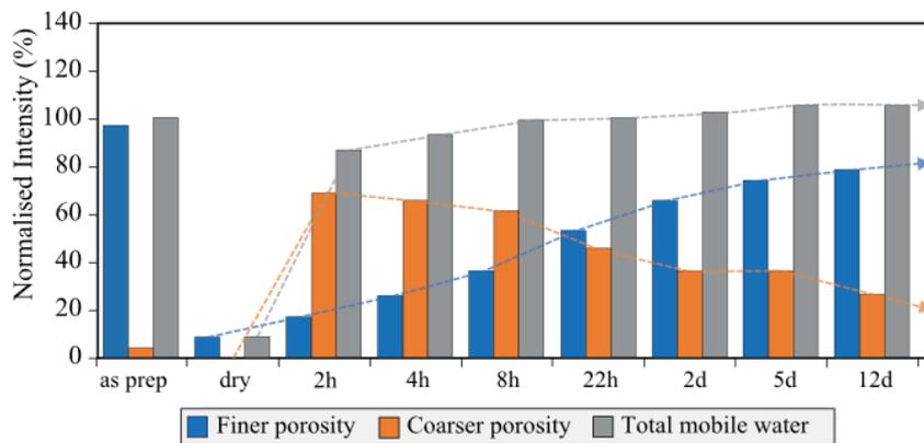
a) Dynamic pore structure of cement-based material during sorption
