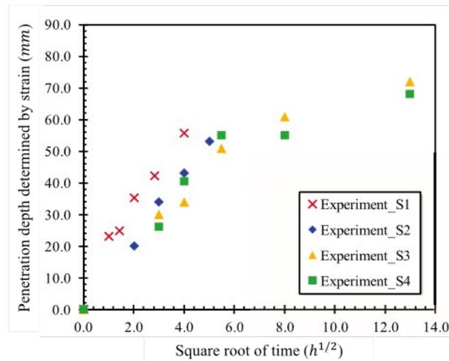
b) Penetration depth development during liquid water uptake
