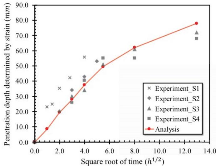
b) Penetration depth development determined by principal strain
