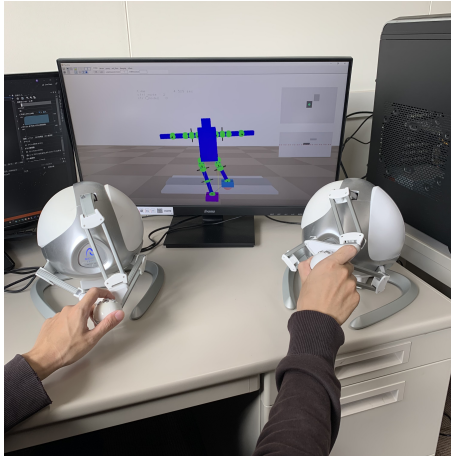
Figure 1. Interactive simulation setup for the step-by-step teleoperation of a humanoid robot.
