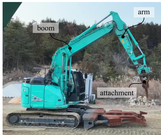
Fig. 12. Kobelco 13-ton class excavator with a shear attachment.
