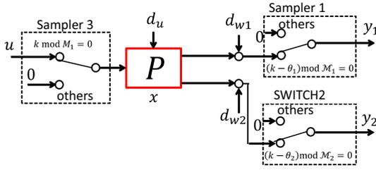
FIGURE 1. Multi-input multi-output plant with different sampling times
