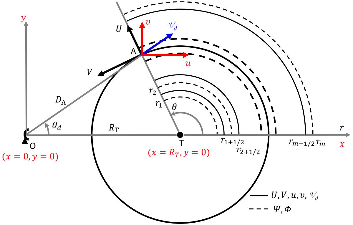
157 FIG. 1. Geometry and symbols in the new approach. A horizontal wind is presented by radial and tangential
