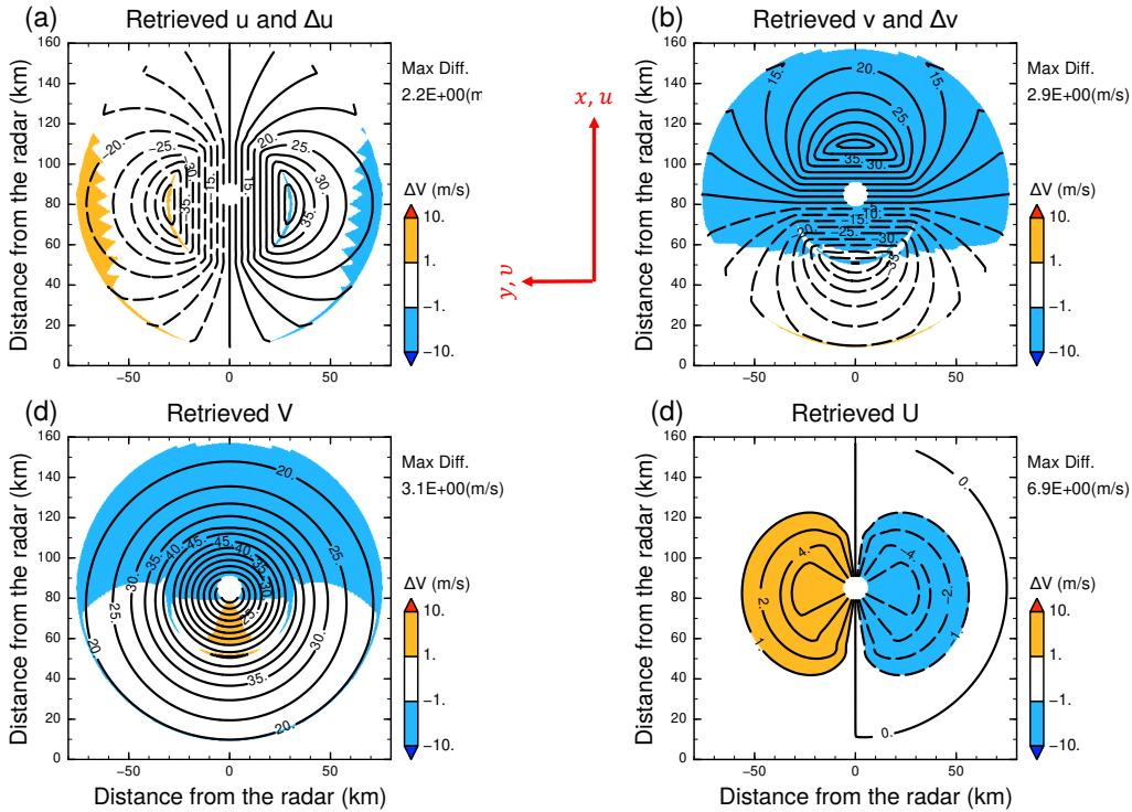
398 FIG. 6. Horizontal distributions of the (a)  $x$ -, (b)  $y$ -, (c) tangential, and (d) radial winds retrieved by GVTD-X
